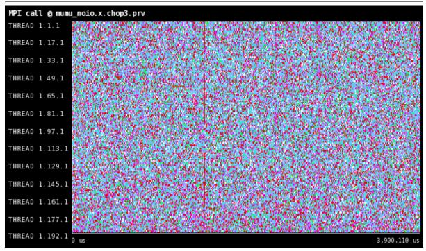
Figure 2: Timeline of a MPI communication phase as seen by Extrae. The duration of this phase is only 3.9 s. It is characterised by some amount of useful user code (shown in light blue) interlaced with large amounts of collective MPI operations, in particular MPI\_Barrier (red) and MPI\_Allreduce (pink).
