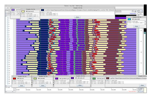
Figure 16: A fragment of the trace of program xx14std, showing MPI routines included directly in the ParaFEM library.
