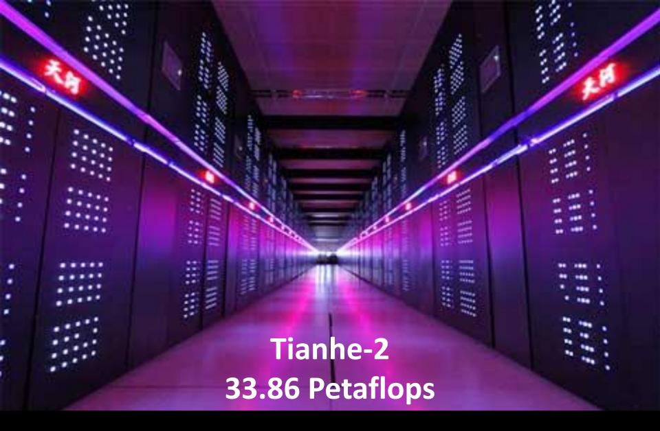
3,120,000 cores (Intel Ivy Bridge and Xeon Phi) 33,860,000,000,000,000 floating point operations per second
