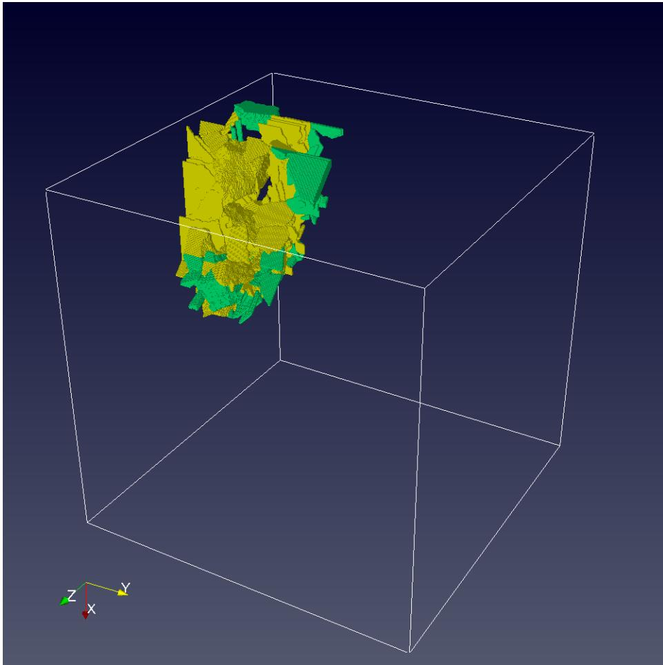
The macro-crack emerges as cleavage cracks in individual grains join up after crossing grain boundaries in poly-crystalline bcc iron. Green cracks - {110} planes, yellow - {100} planes.
